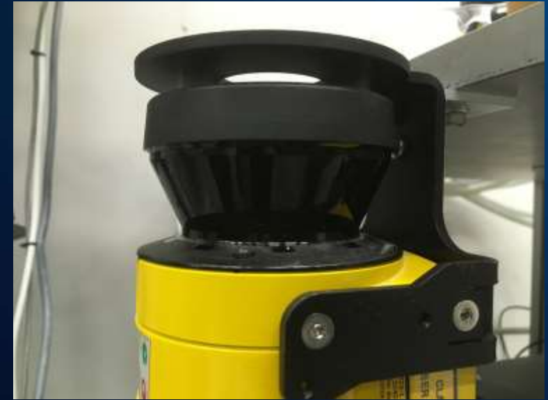
Fig. 2. Example of horizontal mounting of a safety scanner using a protective mounting kit.
