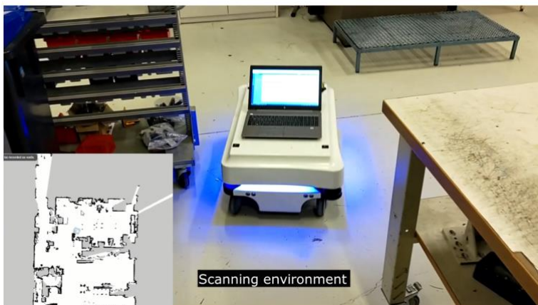
Figure 4: Illustrating the recording of a new map and how to stop it.
